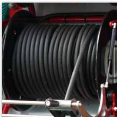
80m. 1/2" (ND13) sewer-jetting hose instead of 50m.
