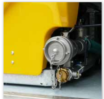
Storz coupling for quick filling of the water tank (optional)
