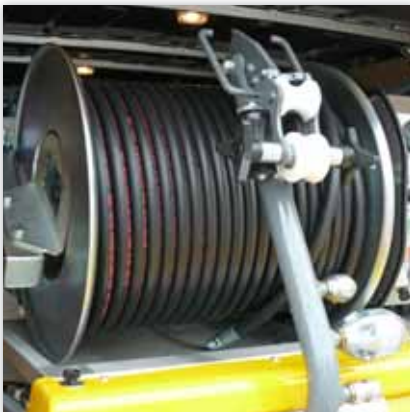
120m. instead of a 80m. 1/2" ROM sewer jetting hose
