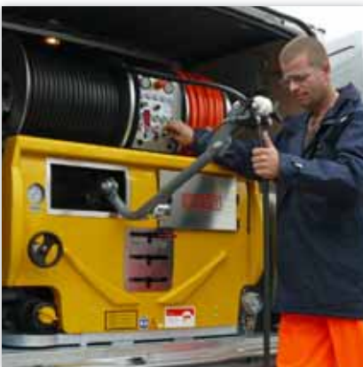
High pressure reel, incl. hose guiding system
