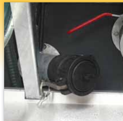
Fixed ventury-type ejector for filling the tank with surface water
