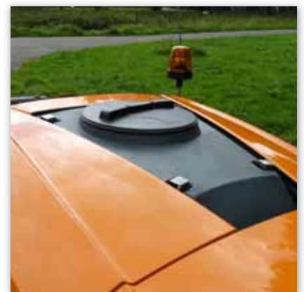
Polyethylene water tank cover with snap-lock seal
