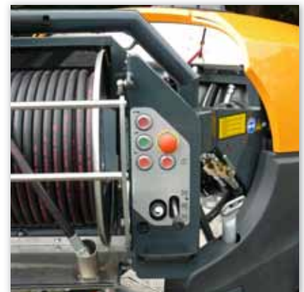
Second control panel swinging out with HP reel, mounted at an ergonomic working height
