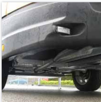
Fully hot dip galvanised chassis
