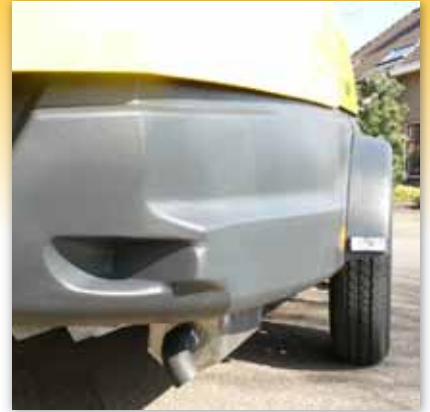
Impact-resistant covers and bottom panels – scratches and tears are easy to repair
