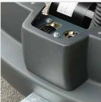
Bonnet catch with unlocking handle in the toolbox
