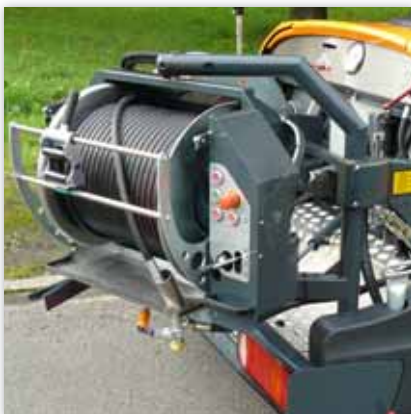
Hydraulically driven HP reel, 270° rotational, lockable at any angle
