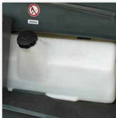
Transparent fuel tank with convenient filling opening
