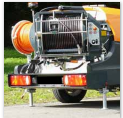
Support legs – extra security for hydraulic reeling of the HP hose
