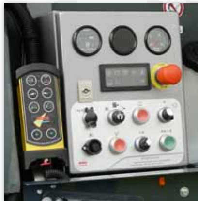
Control box / electronics mounted in lockable, vandalism and water-resistant toolbox
