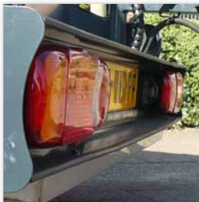
Integrated lighting units protected in the bumper
