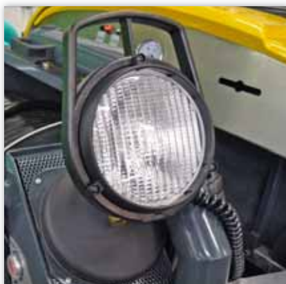
Working light with magnetic bracket
