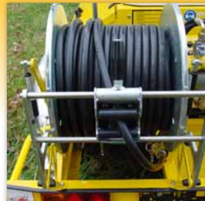
Hydraulically driven HP reel incl. hose guiding system
