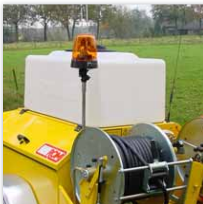
Rotating beacon on extending pole
